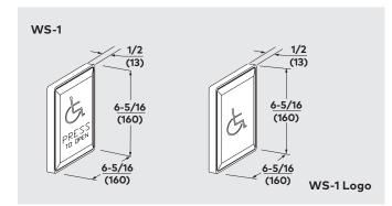
WS-1 — Tamper-resistant 6" × 6" wall plate with a normally open switch. Includes a heavy duty injection molded black ABS mounting box. Satin stainless steel wall plate with blue engraving. Wall plate displays the accessibility symbol and "PRESS TO OPEN." Fits a standard 4" × 4" electrical box. Must be hard wired. Flush design allows the optimum in weather resistance, in surface, or recessed applications.
