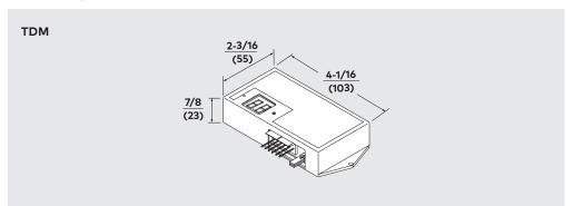
TDM — Advanced time delay module, allowing the installer to use only one time delay for any automatic door operation, on electrically or magnetically locked doors. TDM is required for vestibule sequencing and simultaneous triggering of (2) ED900 operators.
