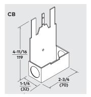
**CB** — UL approved conduit box accessory to provide surface wiring of 120 VAC power to ED900.
