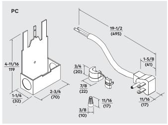
**PC** — Eliminates need for hard wiring. Permits ED900 to plug directly into 120 VAC/60 Hz receptacle. Cord measures 15" from end cap to center of plug.
