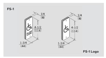
**F5-1**—1-3/4" × 4-1/2" frame plate with a normally open switch. Satin stainless steel frame plate with blue engraving. Frame plate displays the accessibility symbol and "PRESS TO OPEN." Fits a minimum 1-3/4" × 4" frame section. Must be hard wired.
