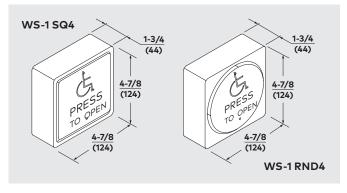
WS-1 SQ4 — Tamperresistant 4-1/2" × 4-1/2" wall plate with a normally open switch. Includes a heavy duty injection molded black ABS mounting box. Satin stainless steel wall plate with blue engraving. Wall plate displays the accessibility symbol and "PRESS TO OPEN." Fits a standard 4" × 4" electrical box. Must be hard wired. Flush design allows the optimum in weather resistance, in surface, or recessed applications.
