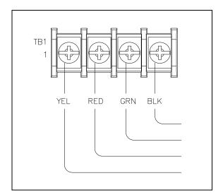
Figure 4. TB1 Terminal Block on Industrial Telephone PCBA
