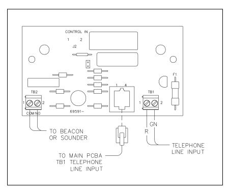
Figure 5. Ring Relay PCBA Wiring
