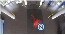
**"U-Turn":** In case MxAnalytics detects an object that deviates from the defined main direction axis in an angle of in between 135° and 180°, this change is interpreted as U-turn and an event is triggered.
