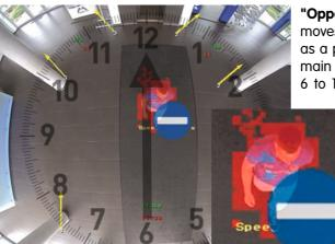
"Opposite Direction": An event is triggered when an object moves opposite to the defined main direction. This direction is set as a position of the clock face. In the example image shown, the main direction "12 o'clock" corresponds with the black arrow from 6 to 12 o'clock or from bottom to top. The person in the image
