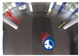
"Duration of Stay": Whenever a detected object stays or moves within the image longer than the defined maximum duration of stay (values between 1 and 300 seconds), an event is triggered. For optimum detection results constant lighting conditions are decisive (ideal: artificial light, no shadows). With direct sun and diffuse shadows it is in most cases only possible to detect durations of stay of a few seconds reliably. The "Duration of Stay" is not suitable for left-luggage detection.
