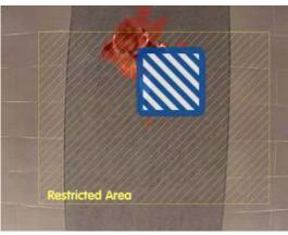
"Restricted Area": With camera firmware version MX-V4.4.0.31 or higher an event can also be triggered if something enters a "digitally marked," rectangular restricted area within the image. Up to 20 different restricted areas can be activated simultaneously for each camera by creating multiple profiles. Active restricted areas can be hidden or made visible within the image by selecting the desired color and transparency.
