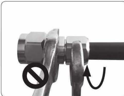
10. Tighten connector body firmly using the two wrenches as shown
