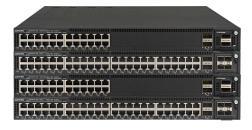
To complete the solution, The ICX 7550 Series includes four Gigabit Ethernet models, two with PoE support and two without. These models come in 24- and 48-port versions and can stack with the rest of the ICX 7550 series to offer traditional Gigabit ethernet connectivity for legacy Wi-Fi access points, VoIP phones, printers, laptop and desktop computers.
