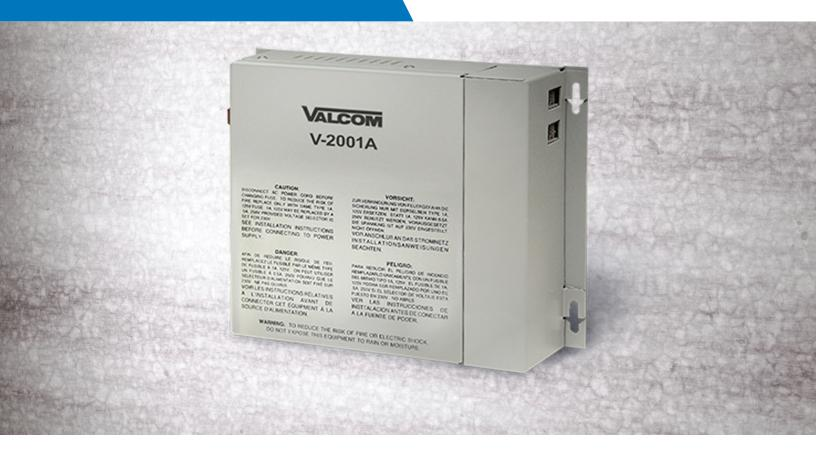
The Valcom V-2001A is a one zone basic integrated page control unit. The V-2001A has a power supply and built-in tone generator for night rings and time clock tones. The V-2001A also enables you to do emergency page overrides for priority announcements.
