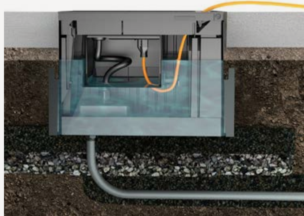
Its NEMA 6P & IP68 Rated "diving bell" design traps and maintains an air pocket, keeping connection points safely away from wet weather.
