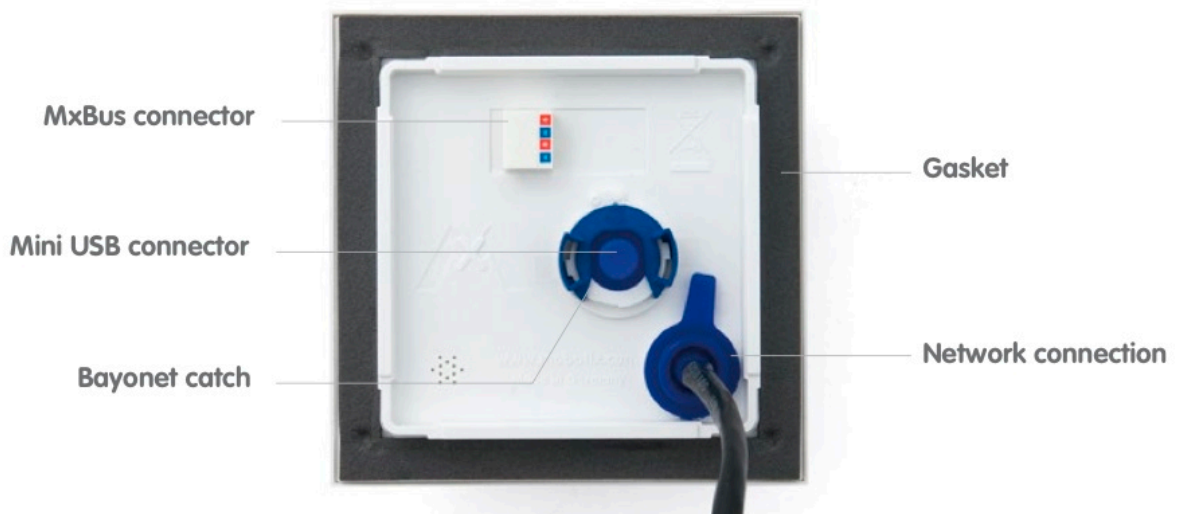
(T25 – Camera housing and connectors, excerpt from the technical documentation)
